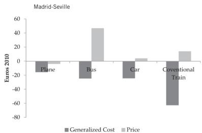
Figure 8.3 Generalized cost and price differential of HSR with respect to other transport modes (e.g., HSR-car)
