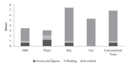
According to Figure 5.1 the faster way to travel between Madrid and Seville is by air. Door-to-door travel time is shorter, though the comparative advantage rests on the substantially shorter invehicle time as the access-egress and waiting time are higher when the airport infrastructure is involved. This is quite interesting because the higher values of access-egress and waiting time leave HSR in a better position when door-to door travel-time costs is the reference (Figure 5.2).
